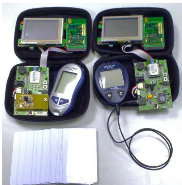
Fig. 5 Movital with LCD color touch screen, RFID reader with some Desfire Mifare cards, and glucometer connected through RS232 (right) and IrDA (left)
