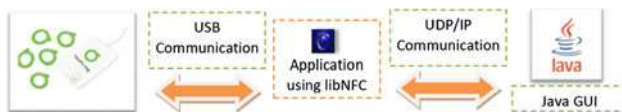
Fig. 7 Application bridge between RFID reader, accessed through LibNFC based on C, and the nurse/physician diabetes management application based on Java
