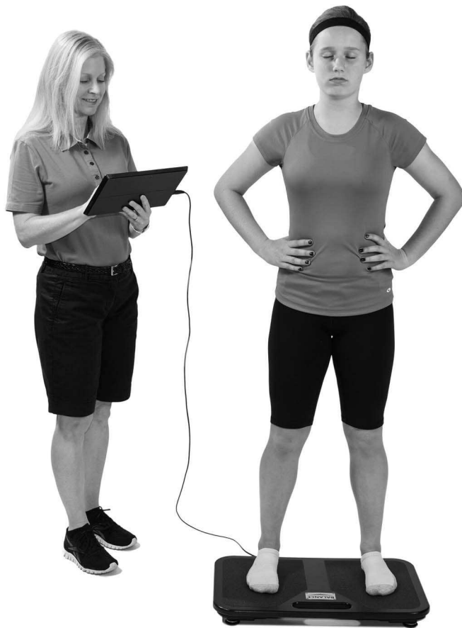
Figure 2. A depiction of the typical BBT administration. The athlete quietly stands wearing socks, on the BTrackS Balance Plate with eyes closed, feet shoulder width apart, and hands on hips while the tester collects COP information on a connected computing device running the BTrackS Sport Balance software. Photograph from http://balancetrackingsystems.com/sport-balance —used with permission.
